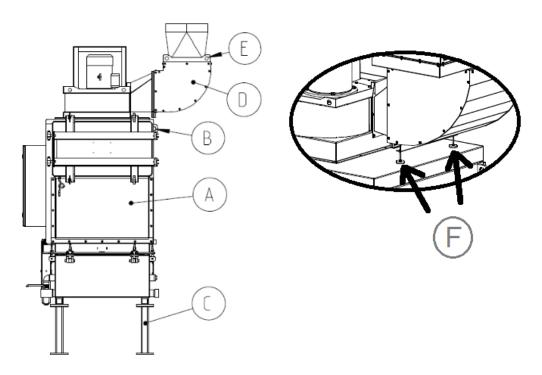
First the filter unit as delivered must be transported to its destination. Then lift the filter unit off the pallet. Therefore use the lifting rings (B).
