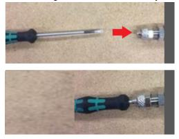
Then re-install the two measuring hoses.
